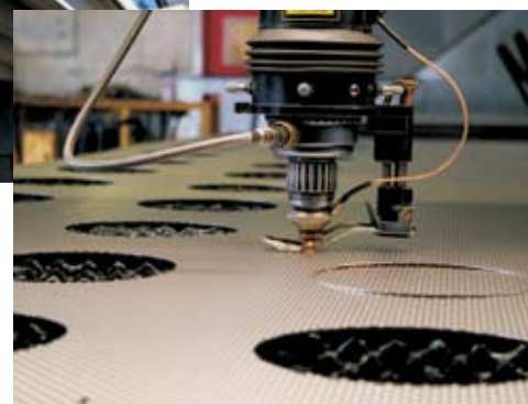
Right: New Touch Laser in Bayswater, VIC, laser-cut every sheet for the bridges' external cladding according to the designers' plan. Photo: Schulz
